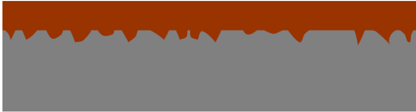
Figure 2 – Illustration of copper laminated to PTFE surface.
